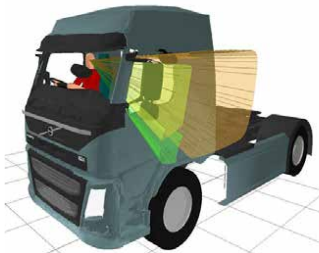
Volumetric projection of driver views through nearside window, illustrating the extent of obstruction caused by mirrors
